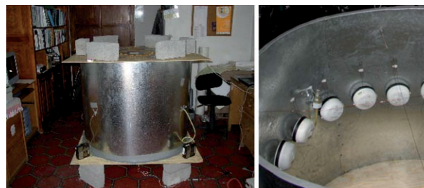
Fig. 1 Test chamber (1.2 m diameter × 1 m height) set up in Mexican field station showing placement of UCBs and cyclone during testing.
